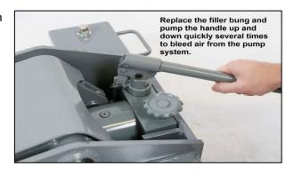
6. Recheck the hydraulic oil level and refill to 6mm below the fill port if required before replacing the filler bung.
